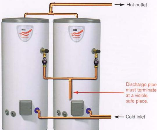
Illustration showing two Megaflow HE in parallel for high usage applications.
